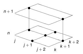
Again we add the integral relations similar to those used for the Laplace Equation and use the trapezoidal integration rule for  $\varphi_x, \varphi_y$  and the midpoint rule for  $\varphi_t$ .
