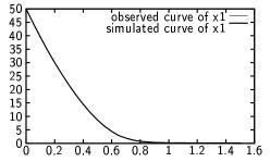
The Levenberg-Marquardt method ends in a wrong local minimum
