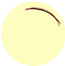
Figure: Crack scenario b_1^* revisited: \delta = 20\% and N = 16 . Reconstruction results for distinct current patterns.
