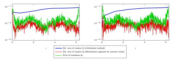
The rotation is around the moving axis  $(\sqrt{1-a^2}\cos(b\sin(t/2)), \sqrt{1-a^2}\sin(b\sin(t/2)), a) \in \mathbb{S}^2$  for a = 0.28 and b = 0.5. The translation is  $d_t = 2(\sin t, \sin t, \sin t)$ . Left: cell phantom. Right: Shepp-Logan phantom.
