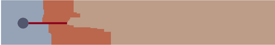
Figure 2: Split configuration using four subdomains. Load balancing issues are obvious.
