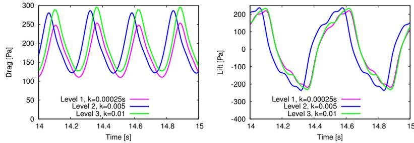
**Fig. 8** Comparison of drag (left) and lift (right) using the biharmonic MMPDE. Here, we make a rather unusual comparison: refining the mesh level while coarsening the time step size. For the drag and the lift we observed less accurate results (not shown here) for the harmonic and elastic MMPDE - in particular when the beam has its largest deformations.
