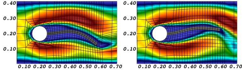
**Fig. 3** Velocity field and mesh deformation at two snapshots using the harmonic MMPDE. The displacement extremum is displayed at left and a small deformation is shown at right. These two time instances also refer to Table 1, where the respective Newton iterations are measured.
