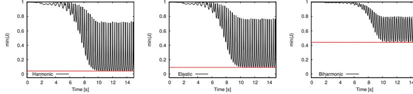
**Fig. 5** Comparison of the mesh regularity for level 1 and  $k = 0.01s$  in terms of  $\min(\hat{J})$  for nonlinear harmonic, nonlinear elastic and linear biharmonic mesh motion.
