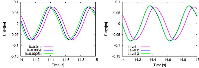
**Fig. 7** Comparison of  $u_y$  using the biharmonic MMPDE. On the left a zoom-in for temporal convergence (on Level 1) is shown and on the right spatial convergence for  $k = 0.01s$  is plotted.
