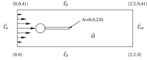
**Fig. 2** Flow around cylinder with elastic beam with circle-center  $C = (0.2, 0.2)$  and radius  $r = 0.05$ .
