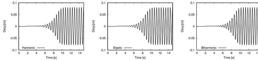
**Fig. 4** Comparison of the  $u_y$  for nonlinear harmonic, nonlinear elastic and linear biharmonic mesh motion on mesh level 1 and  $k = 0.01s$ .
