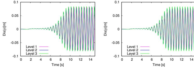
**Fig. 6** Comparison of  $u_y$  for a fixed time step size  $k = 0.01s$  and three different mesh levels. On the left the nonlinear harmonic MMPDE is shown and on the right the biharmonic model.
