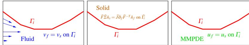
**Fig. 1** Illustration of the three coupling conditions on  $\Gamma_i$  (respectively its corresponding definition on the fixed  $\widehat{\Gamma}_i$ ):  $v_f$  is required to solve the fluid system,  $\widehat{F}\widehat{\Sigma}_s\widehat{n}_s$  is required for the solid system, and  $u_f$  is necessary for solving the MMPDE (fluid mesh motion).
