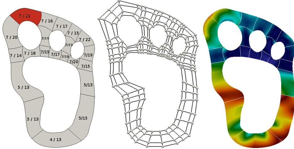
**Fig. 3.** The yeti footprint domain, parameterized by 21 quadratic B-spline patches. Patch segmentation (left), control grids (middle) and the (absolute) Jacobian determinant are shown. On the left picture  $\text{rank}(\det \nabla G)$  and  $\max(\text{rank}(q_{k,\ell}), k, \ell \in \{1, 2\})$  are given.
