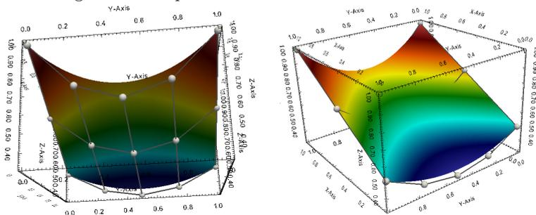
**Fig. 2.** Two views of the graph of the Jacobian determinant and its control grid over the parameter domain  $[0, 1]^2$ . The degree is 2 in the first direction and 4 in the second one.
