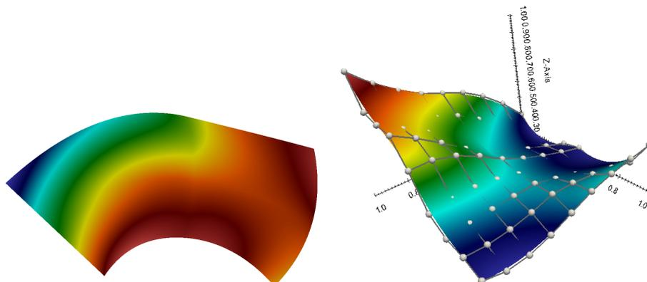
**Fig. 4.** The Jacobian determinant values of the selected patch (Fig. 3) on the domain (left). The graph and control net in parameter domain (right).
