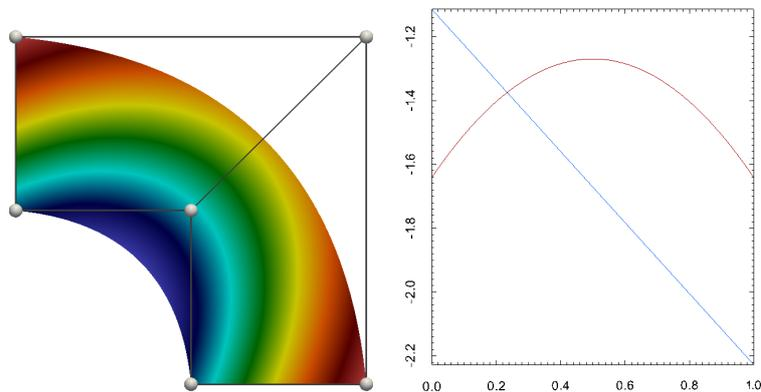
**Fig. 1.** Left: A B-spline quarter annulus domain. The color field is the value of the Jacobian determinant. Right: “Skeleton functions” of the Jacobian determinant. The linear function is associated with the first direction, while the curved one describes the determinant along the second parametric direction.
