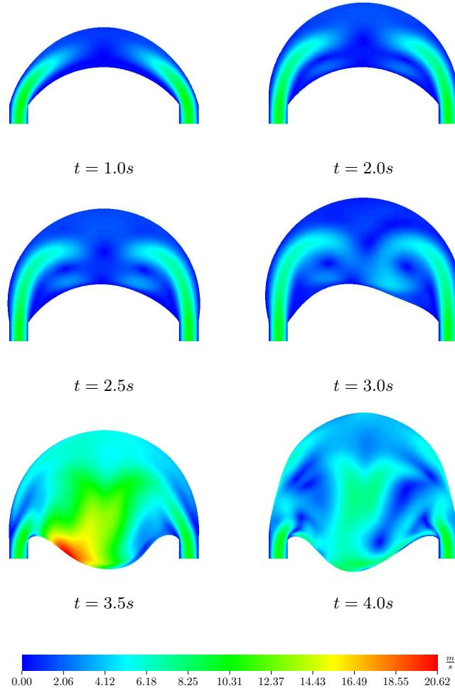
**Fig. 3.** Fluid velocity  $|\mathbf{u}|$ . The structural part is not shown.
