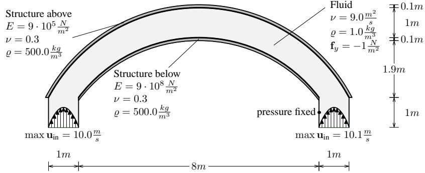
**Fig. 1.** A bended fluid domain with two inflow boundaries constraint by structures of different stiffness.
