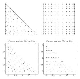
**Fig. 1.** Top: Triangle-Fekete and quadrilateral-GLL points (N=12), Bottom: Triangle-Gauss and quadrilateral-Gauss mapped points (M=19)
