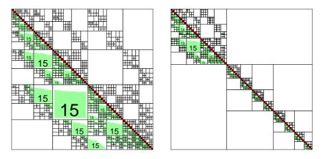
**Fig. 4.**  $\mathcal{H}$ -Cholesky factors of the global stiffness matrix  $A_{\varepsilon}$  (**left**) and of the block matrix  $W_2$  (**right**). The dark blocks  $\in \mathbb{R}^{36 \times 36}$  are dense matrices, the gray blocks are low-rank matrices and the white blocks are zero ones. The steps in the grey blocks show the decay of the singular values in a logarithmic scale. The numbers inside the subblocks indicate the local ranks.
